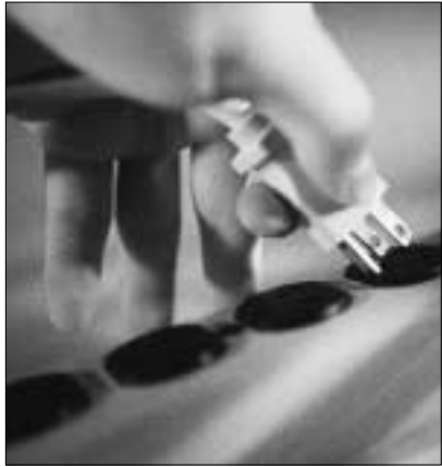
When disconnecting an extension cord, always pull from the plug, never the cord itself.
