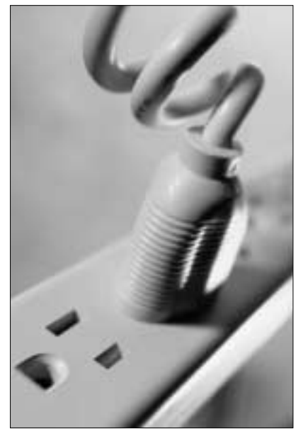
When disconnecting an extension cord, always pull from the plug, never the cord itself.
